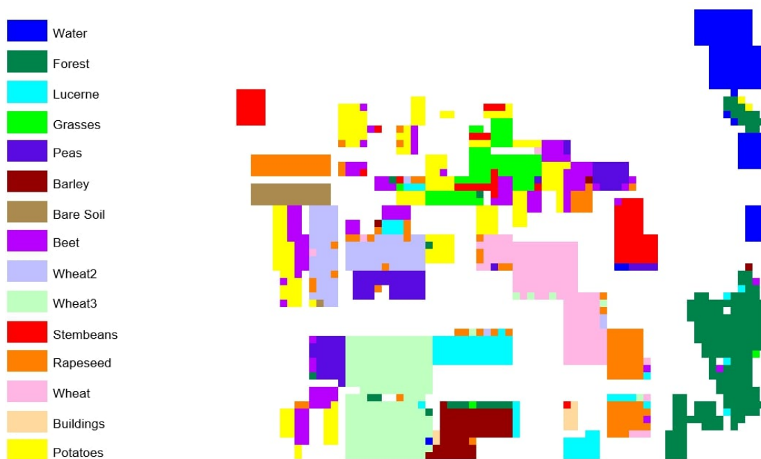
Figure 5.15: Resulting image of Flevoland 15 dataset with Data Augmentation using GCT model ( c=3 ) with the best performance with skip connections
