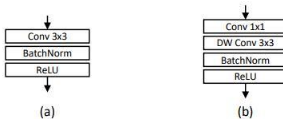
Figure 4.1: (a) Standard 3 × 3 convolution. (b) Lite 3 × 3 convolution. DW: Depth-Wise.[33]
