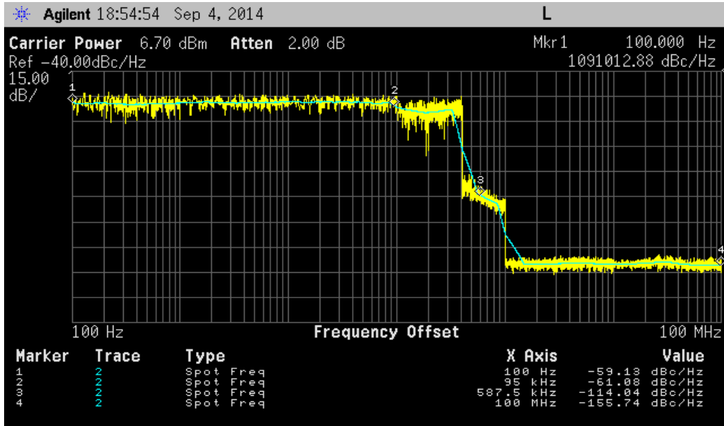
Fig. 5.7. Measured phase noise at 8V varactor bias
