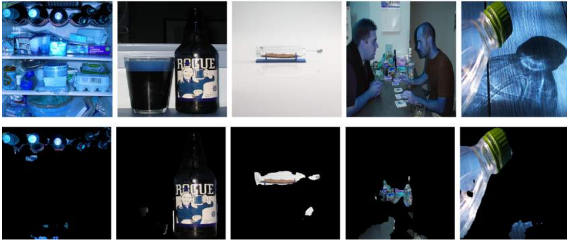
Figure 4.4: Segmentation results for 5-image input to the proposed model trained on image group of size 4 of PASCAL-VOC 2012 [7] data
